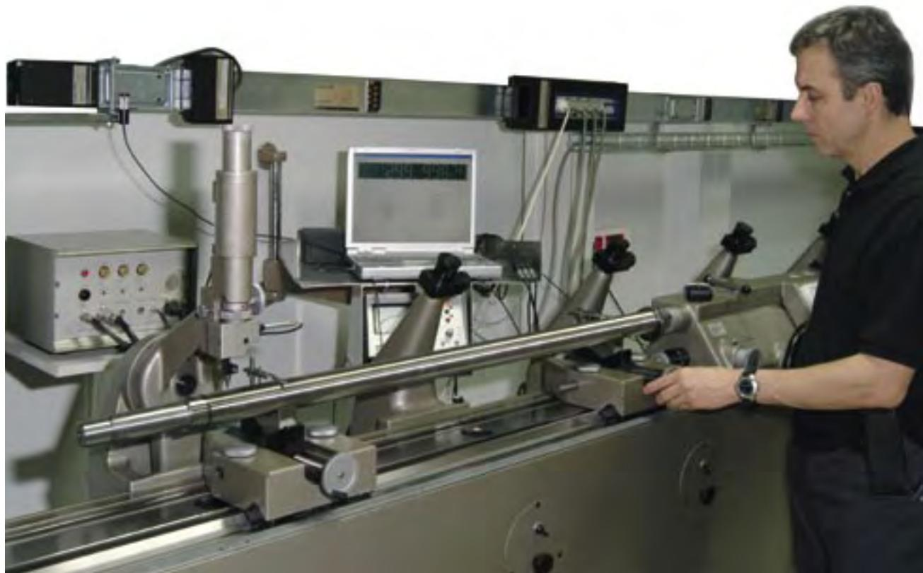
*Lead error control interferometric test bench*
