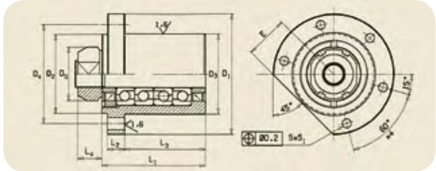
In standard version, the "FLRBU" thrust bearing unit is assembled according to drawing page 30 or 31. If you require a different assembly, please indicate it when ordering.
