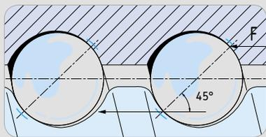
In ball screws, the load is transmitted from the nut to the shaft through the balls engaged in the groove.
