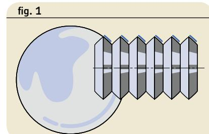
Grooved rollers are the basis of SV/BV/PV recirculating roller screws.
