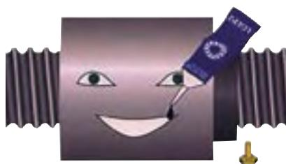
The volume, spread and frequency of the application of the lubricant (oil or grease) must be properly selected and monitored. At high speed the lubricant spread on the surface of the screw shaft may be thrown off by centrifugal forces. It is important to monitor this phenomenon during the first run at high speed and possibly adapt the frequency of re-lubrication or the flow of lubricant, or select a lubricant with a higher viscosity.
