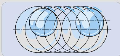
In roller screws, the load is transmitted from the nut to the shaft through the barreled surfaces of all the engaged rollers.
