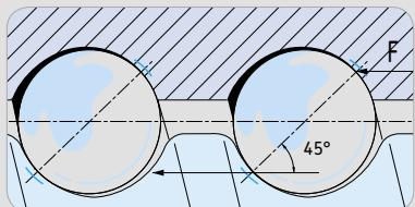
In ball screws, the load is transmitted from the nut to the shaft through the balls engaged in the groove.
