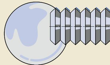
Grooved rollers are the basis of SV/BV/PV recirculating roller screws.
