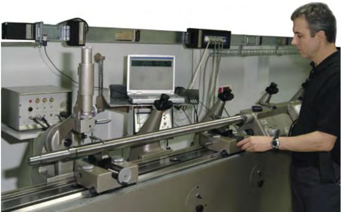
*Lead error control interferometric test bench*
