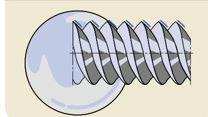
Threaded rollers are the basis of SR/BR/TR/PR planetary roller screws.
