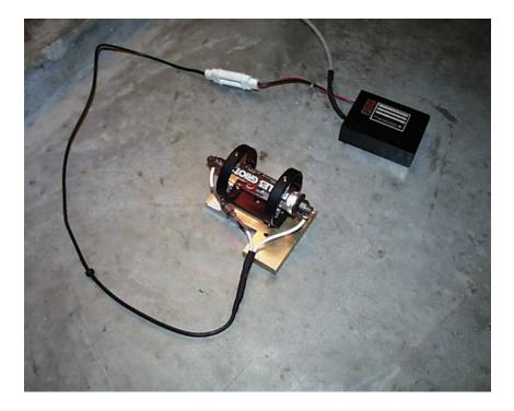
37) After you have the above items sorted out, place the two lasers on a hard flat and stable surface about 5 ft (1.5 meters) apart with the beam from the alignment laser facing the Output End of the CO2 Laser.
