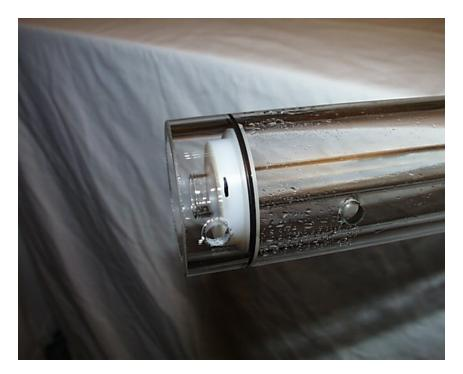
At the total reflector end, the bore tube should be inserted exactly  $\frac{1}{2}$ " or 12.7 mm into the cooling jacket, and the bore mount should be inserted 5/8" or 15.8 mm. It is very important that the bore protrudes a minimum of 1/8" or 3.2 mm from the Nylon bore support at this end.
