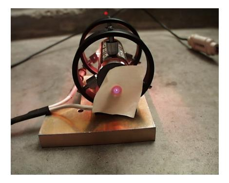
39) Take another piece of masking tape with a tiny hole (~2mm) punched in it's center (See above technique), and apply it over the hole in the center of the Brass End Cap, at the output end of the tube. The hole in the tape should be aligned as precisely as possible with the center of the bore.
