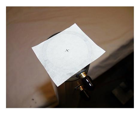
41) Carefully align the HeNe laser so that the beam is exactly centered on the small hole in the tape at the front of the CO2 Laser, and then passes down the length of the CO2 Laser Tube and strikes the last piece of masking tape exactly in the center of the bore where you marked an X. What you should now have is the HeNe laser beam aligned so that it passes directly through the exact center of the CO2 Laser bore tube.
