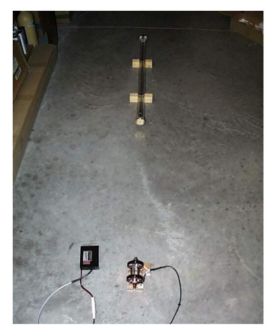
38) Use a piece of masking tape with a tiny hole punched in it to cover the front of the alignment laser. Align the tape so that the beam is coming through the center of the small hole. The hole should be roughly the same size as the beam and centered on the beam.
