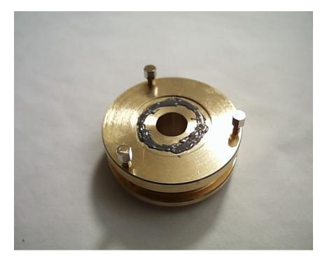
29) Insert the "Rear Mirror" along with its Phenolic Insulator into this "Adjustable Rear Cell" and press well into place rotating to spread the epoxy in a very thin layer, then set aside to dry for several hours. **DO NOT GLUE THE OUTPUT COUPLER TO THE OTHER BRASS END AT THIS TIME.**
