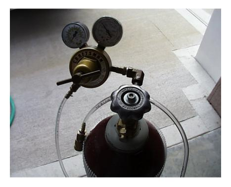
8) Ensure that the flow control valve on the gas flow meter is CLOSED.
