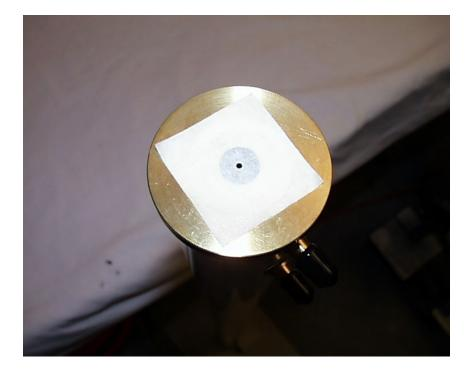
40) Take a third piece of masking tape and apply at the rear end of the CO2 Laser. This piece of tape should not have a hole in it but just cover the end of the tube. Use a ruler to mark a small X at the exact center of the tube on this piece of tape, but do not make a hole in this one.
