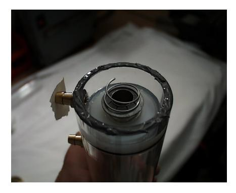
33) Apply a small amount of the epoxy around the inside edge of the lip on the Non Adjustable Brass end.
