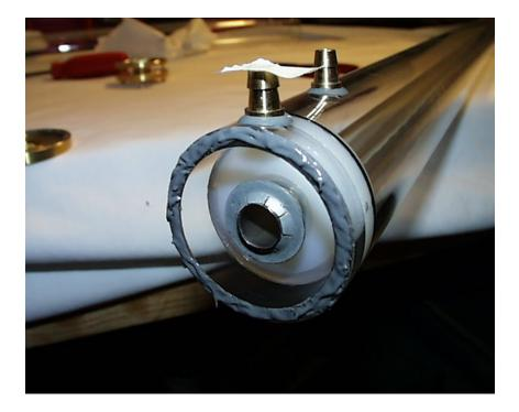
32) Stand the tube upright and place the Cathode Retainer Spring onto the Cathode. Wide section goes toward the Cathode.
