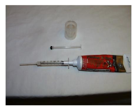
12) Use the syringe to fill the two grooves in each bore mount. Be sure to insert the tip of the syringe all the way to the bottom of the slot, and move slowly all the way around being sure to fill the entire groove as you go. Excess silicone can be wiped away using your finger tip.
