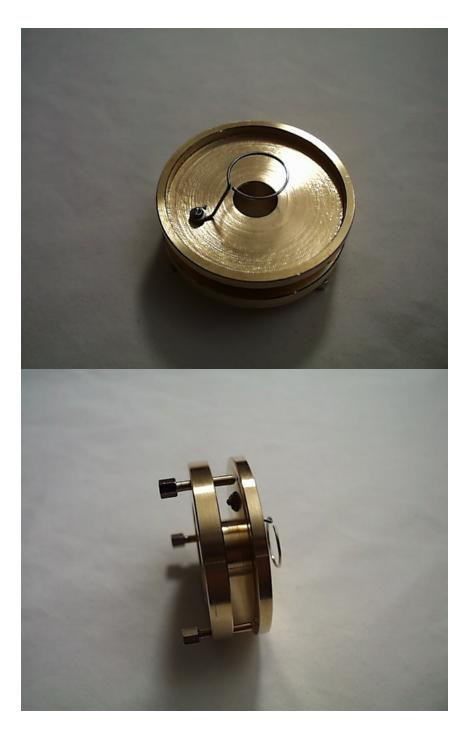
21) Trial fit the Adjustable Brass End onto the cooling jacket to ensure that the Anode attached in the previous step does not interfere with the glass. If it does, loosen the screw and slide the Anode in further, then re-tighten and align as described above. When satisfied, set aside to dry for several hours and continue with the next step.
