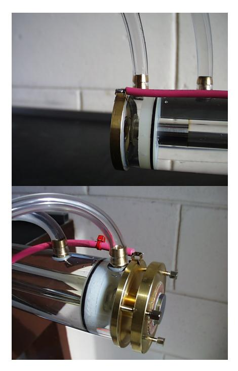
4) Fill the cooling jacket with tap water by slowly opening the ball valve. As the tube fills, tip it so that all air is removed via the overflow line. After the tube is filled with water, set the flow rate to about 2 - 3 liters per minute.
