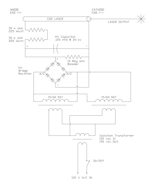
If you are planning to use the laser for CNC cutting or engraving, then the smoothing capacitor should be used to remove the 60 hz output. However,
