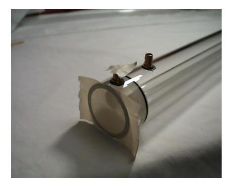
NOTE: It is very important to ensure that all particles of lint and dust have been removed from the tube and the cavities at the ends. Failure to do so will result in the particles being vaporized when the tube is ionized, and could cause damage to the coatings of the mirrors, therefore reducing the life of the tube. Clean the tube well and use plenty of compressed air.
