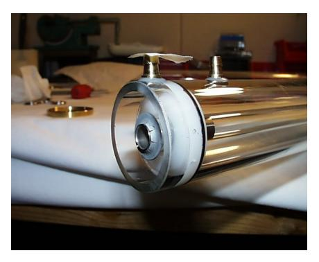
31) Mix up another batch of epoxy and apply a thin layer to the Output End of the glass cooling jacket.
