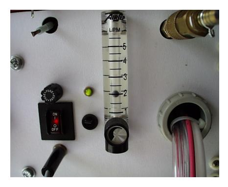
11) Next switch on the high voltage and you should immediately see a purple-blue discharge in the tube. If no discharge occurs, the gas pressure may be too high inside of the tube and you will need to reduce the flow rate slightly until the tube ionizes.
